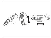
Holding the new toner bottle as shown on the right, pull out the seal in the direction of the arrow.
